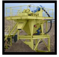
The SPHERIUS F-Range offer sand processing solutions that utilize cyclone, pump and dewatering technology to produce specification sands and are capable of recovering all saleable sand coarser than 40 micron therefore increasing sand production, increasing plant capacity and reducing settling pond maintenance costs.
